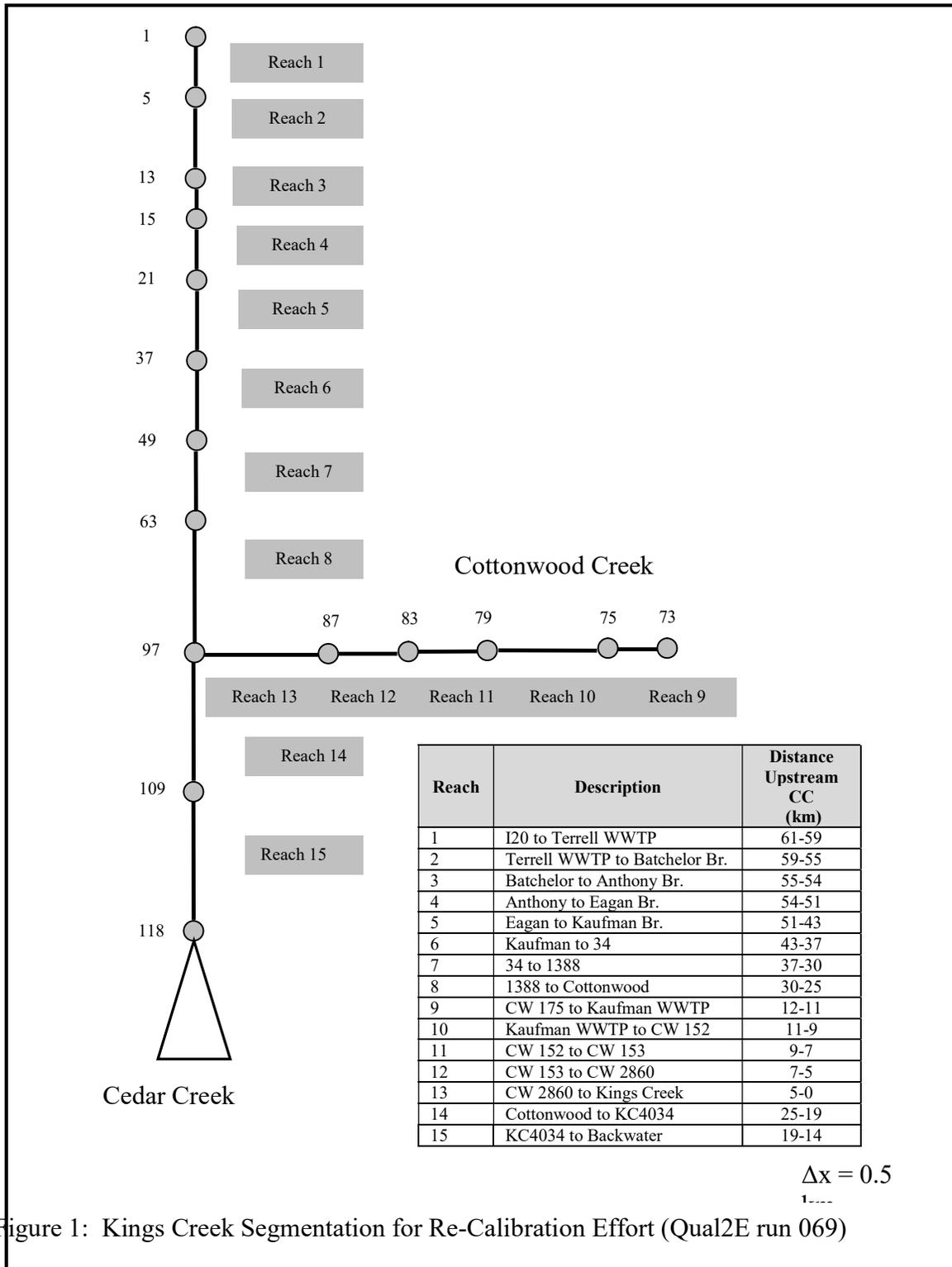
Figure 1: Kings Creek Segmentation for Re-Calibration Effort (Qual2E run 069)
