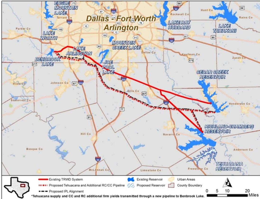
**Pipeline Route to Lake Benbrook (Tehuacana and Richland-Chambers & Cedar Creek Constructed Wetlands Supply in a New Pipeline Parallel to IPL)**
