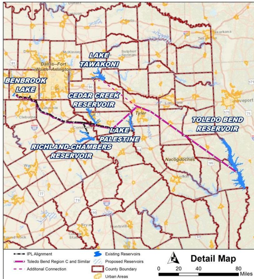
**Figure 4.24 – Proposed Pipeline Route for Toledo Bend Reservoir**
