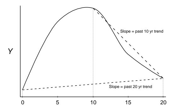
Calculation of rate quantities for complex, cubic trends. The fitted regression model for parameter *Y* is show as the solid curve. The heavy, long-dashed lines show slopes calculated over the past 10 and past 20 years. These slopes estimate the net rates of trend over these time frames. In this case a long term increase is indicated, but must be interpreted in the context of large, more recent decrease.
